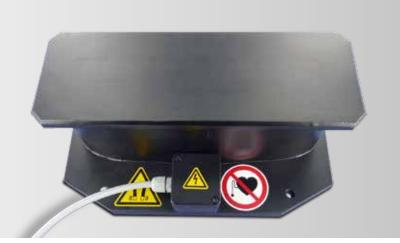
The Portable Demagnetizing Device LIST-MAGNETIK HE-2 can be used either mobile or stationary, as required. The portable device demagnetizes machine parts, tools, rotary parts, cutting plates and much more. It has a 230 V AC connection and produces an alternating magnetic field of 50 Hz with sufficient field strength for the demagnetization of alloyed steels.
